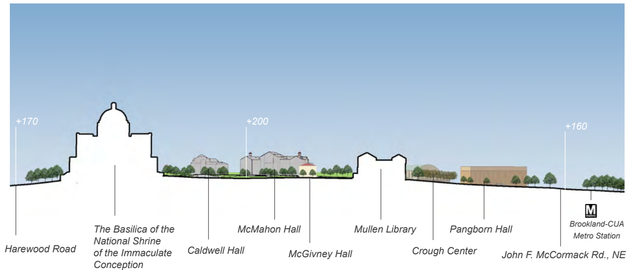
Site Section illustrating grade change from Harewood Road and John McCormack Road to the campus core
